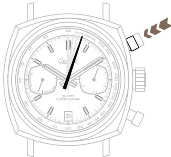
3. To reset the chronograph, press the reset pusher. The chronograph hand will jump back to the 12 position ('instant reset' function).
