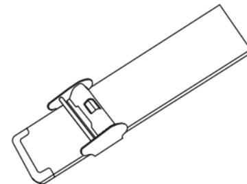
To loosen the clamping mechanism, use a small flat-headed screwdriver or equivalent tool. You can then slide the clasp up and down to find the perfect fit for your wrist.
