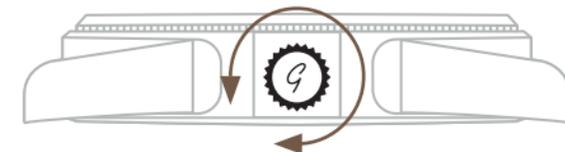
1. First, unscrew the crown until it 'jumps out' slightly into its normal position.
