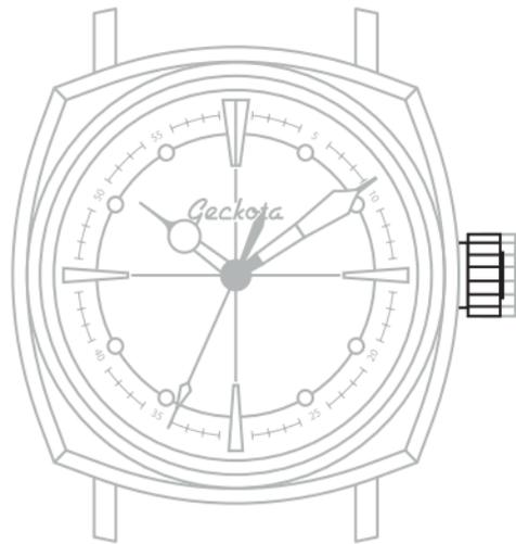
2. Wind the watch by turning the crown CLOCKWISE 20-55 times.
