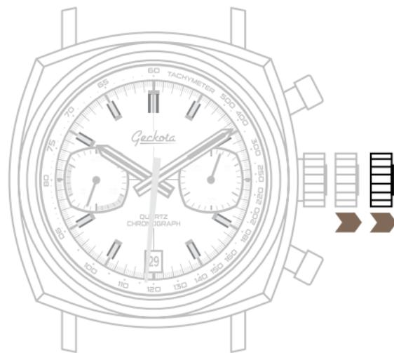
2. Press the reset pusher and hold it down for two seconds. This will return the hands to their correct positions. Then screw down the crown.
