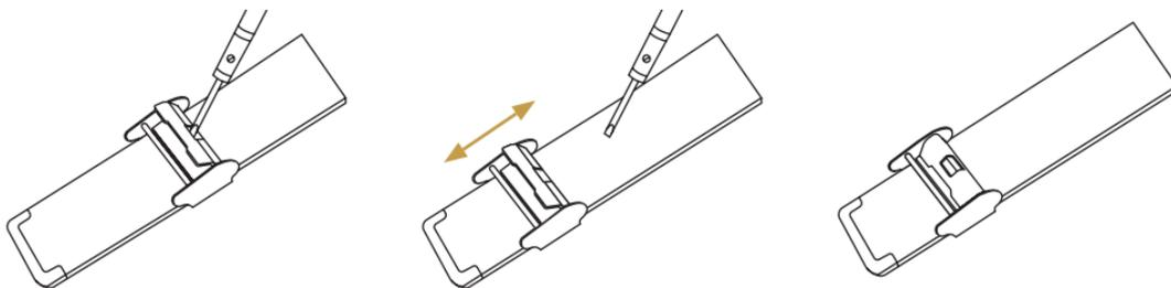
To loosen the clamping mechanism, use a small flathead screwdriver or equivalent tool. You can then slide the clasp up and down to find the perfect fit for your wrist.
